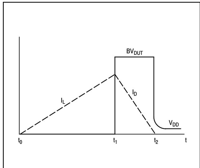
Figure 7. Current-Voltage Waveforms
