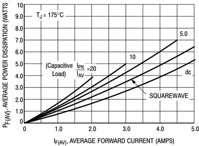
Figure 4. Power Dissipation
