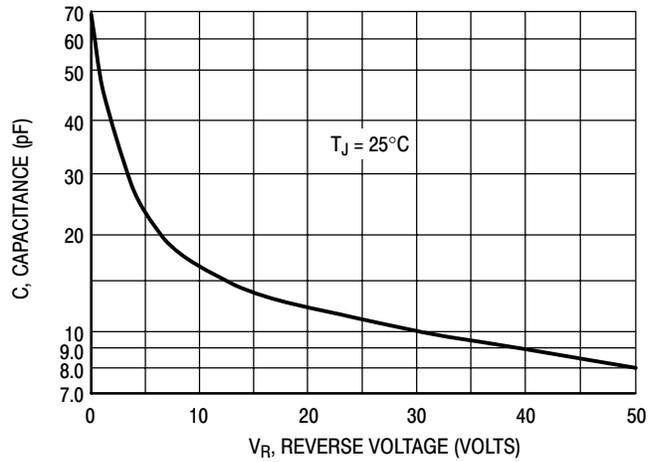
Figure 5. Typical Capacitance
