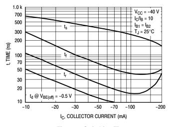
Figure 3. Switching Times
