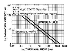
Figure 6. Unclamped Inductive Switching Capability
