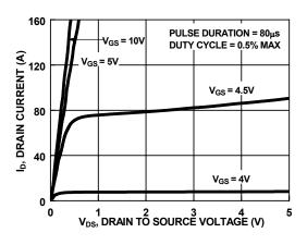
Figure 8. Saturation Characteristics
