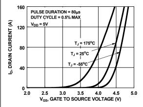
Figure 7. Transfer Characteristics
