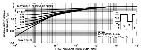
Figure 3. Normalized Maximum Transient Thermal Impedance
