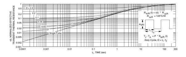
Figure 11. Transient Thermal Response Curve.
