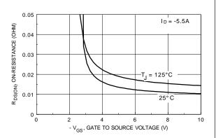
Figure 3. On-Resistance Variation with Temperature.
