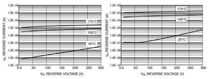
Figure 3. Typical Reverse Voltage
