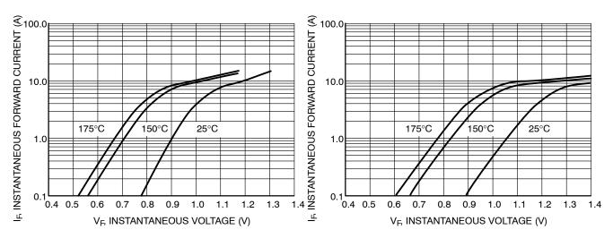
Figure 1. Typical Forward Voltage
