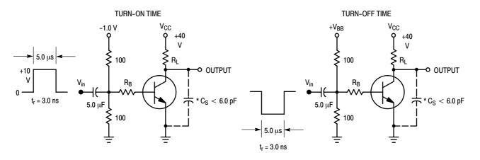
\*Total Shunt Capacitance of Test Jig and Connectors For PNP Test Circuits, Reverse All Voltage Polarities
