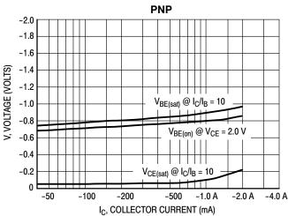
Figure 4. MPS750, MPS751 On Voltages
