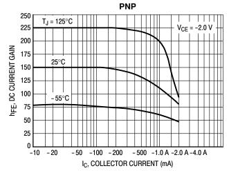
Figure 2. MPS750, MPS751 Typical DC Current Gain
