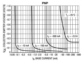
Figure 6. MPS750, MPS751 Collector Saturation Region
