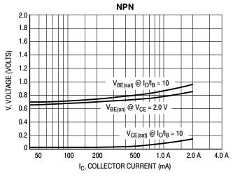
Figure 3. MPS650, MPS651 On Voltages
