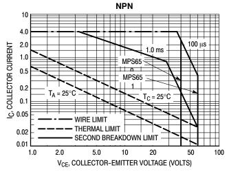
Figure 7. MPS650, MPS651 SOA, Safe Operating Area
