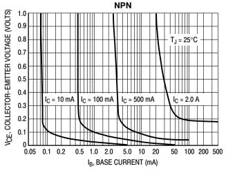
Figure 5. MPS650, MPS651 Collector Saturation Region
