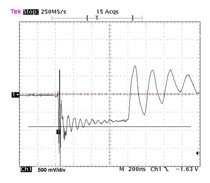
Figure 5. ESD Response for Human Body Model (-8.0 kV)
