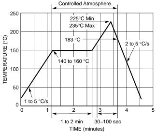
Figure 7. Solder Reflow Profile
