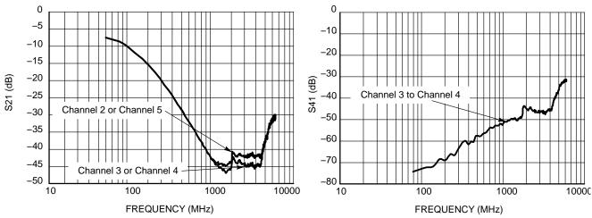
Figure 1. Insertion Loss Curve
