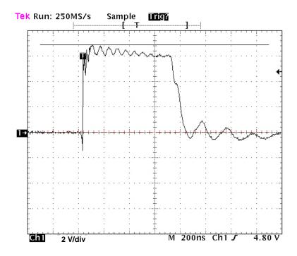
Figure 4. ESD Response for Human Body Model (+8.0 kV)
