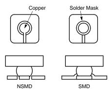
Figure 6. Solder Mask versus Non-Solder Mask Definition
