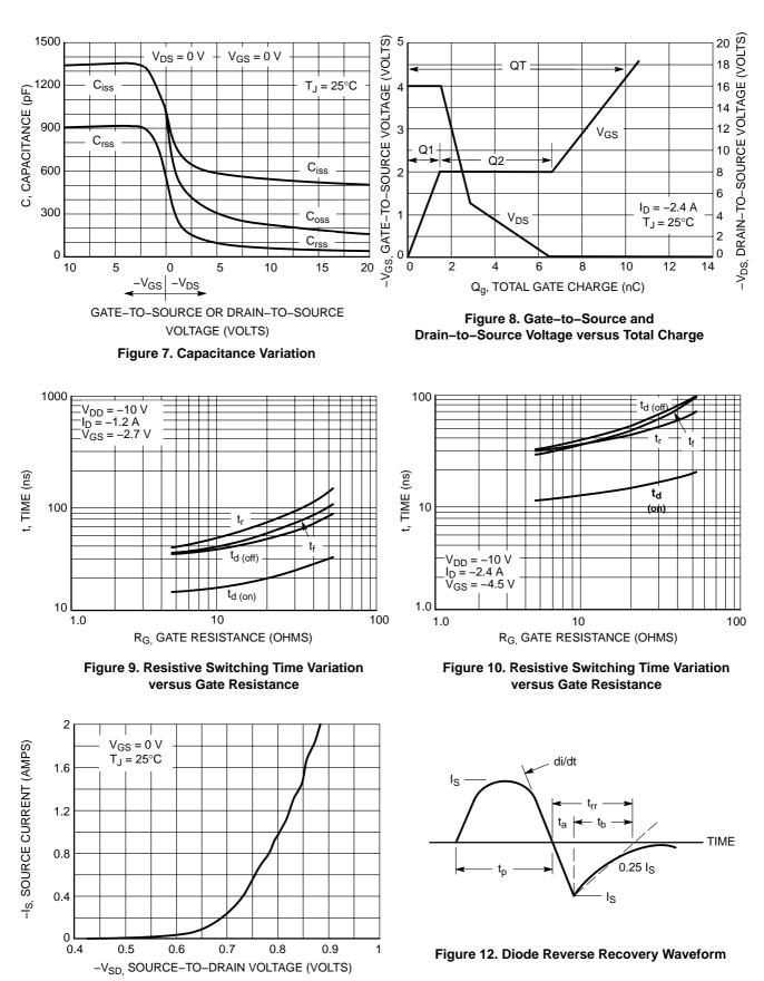
Figure 11. Diode Forward Voltage versus Current
