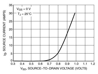
Figure 10. Diode Forward Voltage vs. Current
