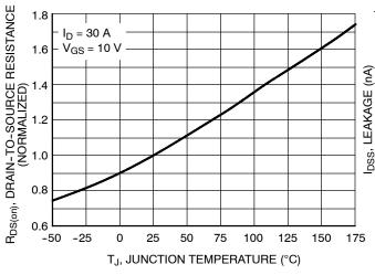
Figure 5. On-Resistance Variation with Temperature
