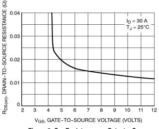
Figure 3. On-Resistance vs. Gate-to-Source Voltage
