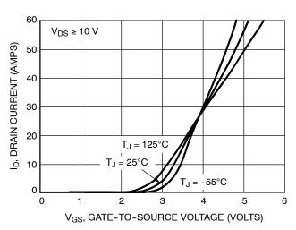
Figure 2. Transfer Characteristics
