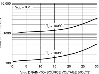
Figure 6. Drain-to-Source Leakage Current vs. Drain Voltage
