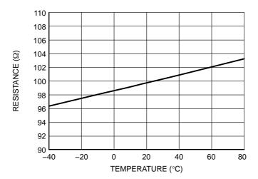
Figure 3. Typical Resistance over Temperature
