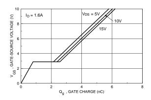
Figure 10. Gate Charge Characteristics.
