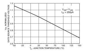
Figure 6. Gate Threshold Variation with Temperature.
