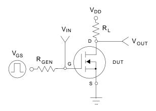
Figure 11. Switching Test Circuit.
