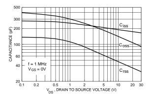
Figure 9. Capacitance Characteristics.
