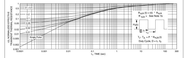
Figure 17. Transient Thermal Response Curve.
