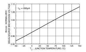
Figure 7. Breakdown Voltage Variation with Temperature.
