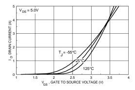
Figure 5. Transfer Characteristics.
