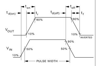
Figure 12. Switching Waveforms.
