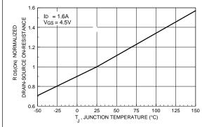
Figure 3. On-Resistance Variation with Temperature.
