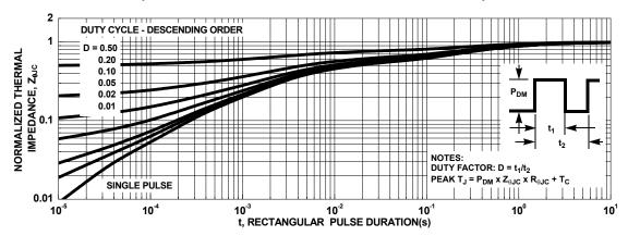
Figure 3. Normalized Maximum Transient Thermal Impedance
