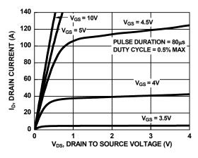
Figure 8. Saturation Characteristics
