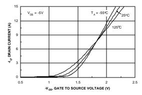
Figure 5. Transfer Characteristics.
