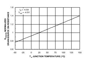
Figure 3. On-Resistance Variation with Temperature.
