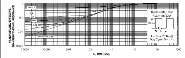
Figure 11. Transient Thermal Response Curve.
