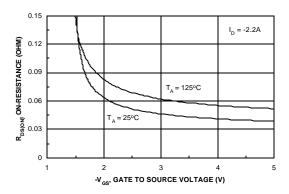
Figure 4. On-Resistance Variation with Gate-to-Source Voltage.
