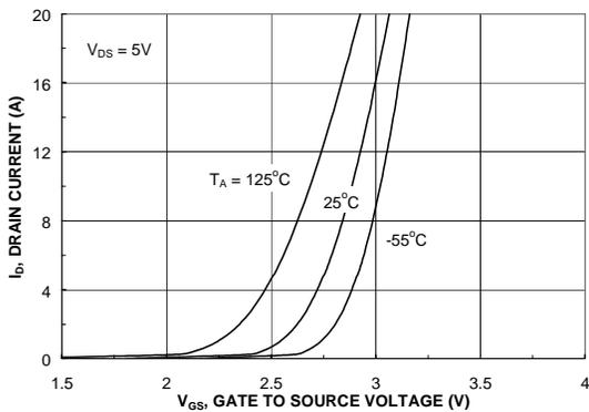
Figure 5. Transfer Characteristics.
