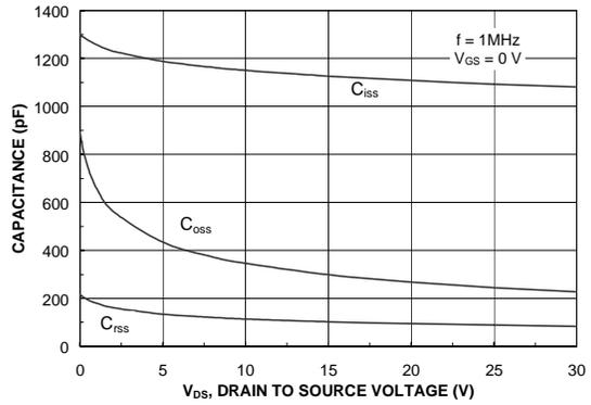
Figure 8. Capacitance Characteristics.
