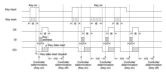
$t5 \, \cdots \, Key$  scan execution time when the key data agreed for two key scans. (615T(s))
