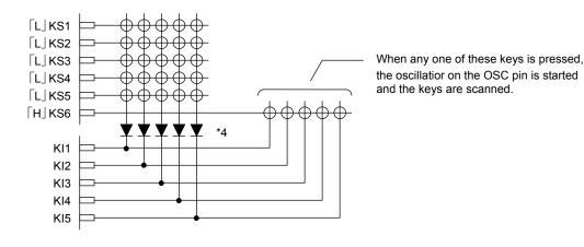
Note: \*4. These diodes are required to reliable recognize multiple key presses on the KS6 line when sleep mode state with only KS6 high, as in the above example. That is, these diodes prevent incorrect operations due to sneak currents in the KS6 key scan output signal when keys on the KS1 to KS5 lines are pressed at the same time.
