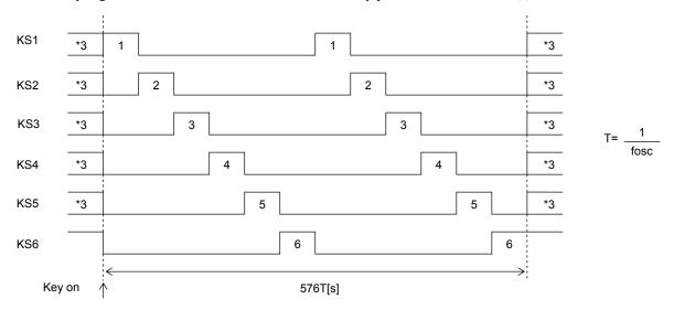
Note: \*3. In sleep mode the high/low state of these pins is determined by the S0 and S1 bits in the control data. Key scan output signals are not output from pins that are set low.
