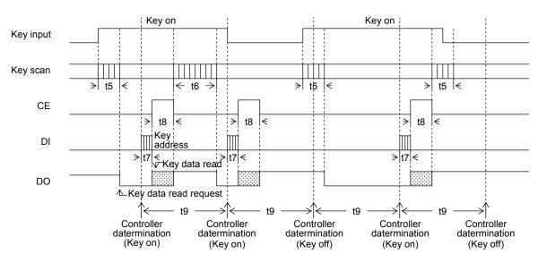
t5 ···· Key scan execution time when the key data agreed for two key scans. (615T(s))
