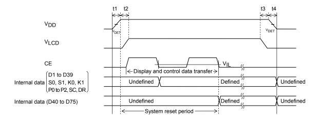
Note:  $t1 \ge 1$  [ms] (Logic block power supply voltage  $V_{DD}$  rise time)
