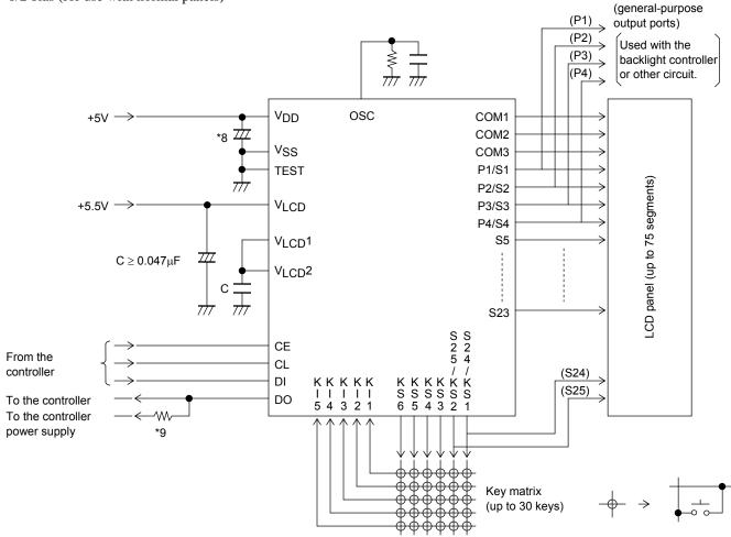
Note: \*8. Add a capacitor to the logic block power supply line so that the logic block power supply voltage V<sub>DD</sub> rise time when power is applied and the logic block power supply voltage V<sub>DD</sub> fall time when power drops are both at least 1 ms, as the LC75863W is reset by the V<sub>DET</sub>.
