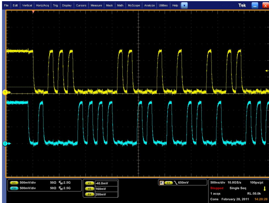
Figure 8. EMI4183 MIPI D-PHY LP Mode Measured Results
