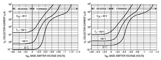
Figure 13. Typical Collector Cut-Off Region
