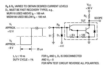
Figure 2. Switching Times Test Circuit
