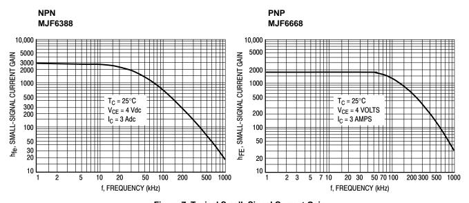
Figure 7. Typical Small-Signal Current Gain
