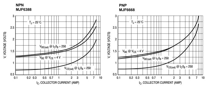
Figure 11. Typical "On" Voltages
