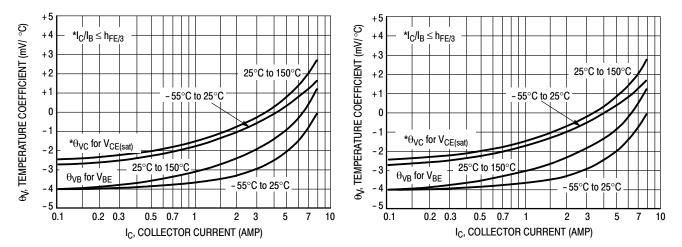
Figure 12. Typical Temperature Coefficients
