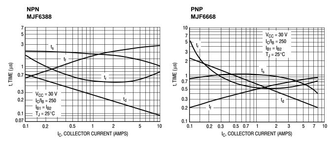
**Figure 3. Typical Switching Times**
