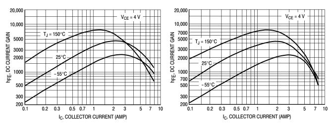
Figure 9. Typical DC Current Gain
