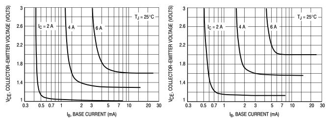
Figure 10. Typical Collector Saturation Region
