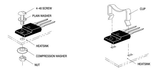
Figure 15. Typical Mounting Techniques\*
