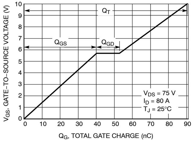
Figure 8. Gate-to-Source Voltage vs. Total Gate Charge
