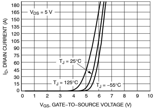
Figure 2. Transfer Characteristics
