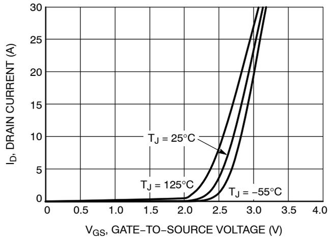
Figure 2. Transfer Characteristics
