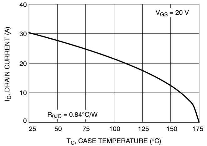
**Figure 10. Maximum Continuous Drain Current vs. Case Temperature**
