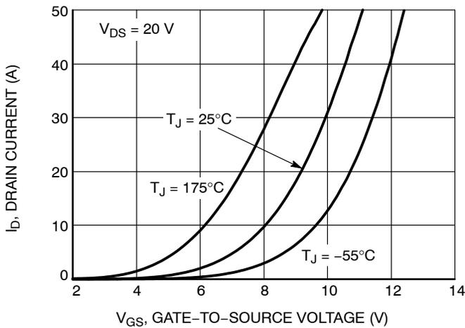
Figure 5. Transfer Characteristics
