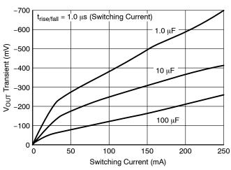
Figure 7. Load Transient Response
