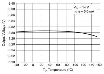
Figure 14. Output Voltage vs Junction Temperature, 3.3 V
