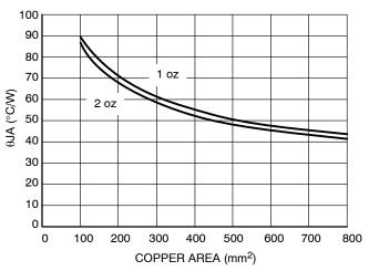
Figure 21.  $D^2PAK$  7-lead  $\theta JA$  as a Function of the Pad Copper Area Including Traces, Board Material
