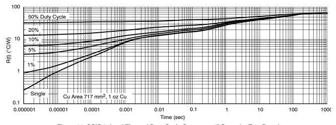
Figure 29. SOIC 8-Lead Thermal Duty Cycle Curves on 1" Spreader Test Board
