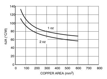
Figure 27. SOIC 8–Lead EP  $\theta$ JA as a Function of the Pad Copper Area Including Traces, Board Material
