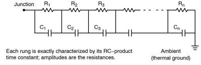
Figure 31. Non-Grounded Capacitor Thermal Ladder ("Foster" Ladder)
