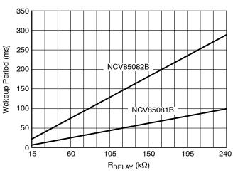
Figure 11. Wakeup Period vs Reset Delay Resistor
