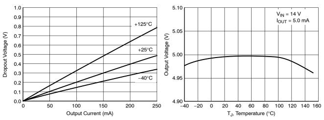
Figure 12. Dropout Voltage vs Output Current
