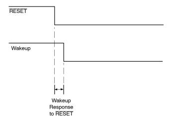
Figure 19. Wakeup Response to RESET (Low Voltage)
