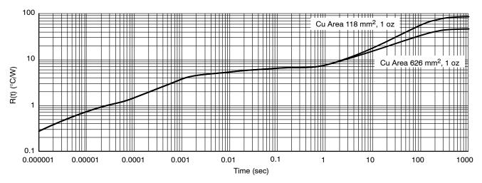
Figure 22. D<sup>2</sup>PAK 7-Lead Single Pulse Heating Curve
