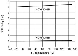
Figure 8. Reset Delay Time vs Junction **Temperature**
