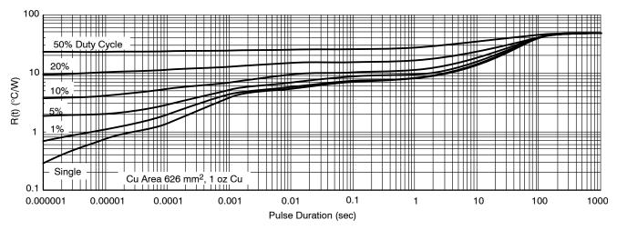
Figure 23. D<sup>2</sup>PAK 7-Lead Thermal Duty Cycle Curves on 1" Spreader Test Board
