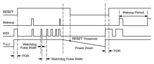
Figure 5. Power Down and Restart Sequence
