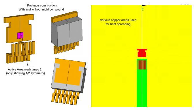
Figure 20. PCB Layout and Package Construction for Simulation
