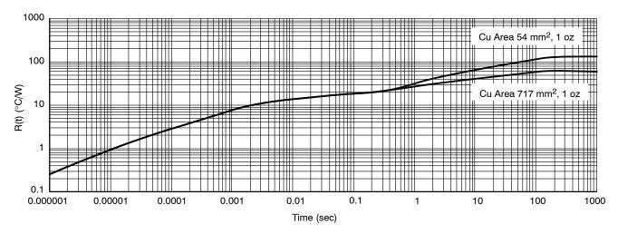
Figure 28. SOIC 8-Lead EP Single Pulse Heating Curve
