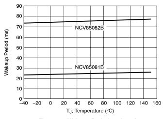
Figure 10. Wakeup Period vs Junction **Temperature**
