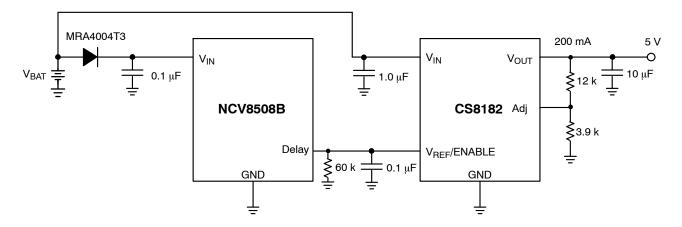
Figure 17. Application Circuit
