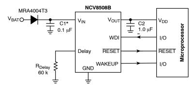
\*C1 required if regulator is located far from power supply filter.
