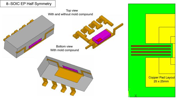
Figure 26. Internal Construction of the Package and PCB Layout for Multiple Pad Area
