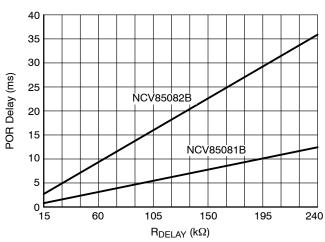
Figure 9. Reset Delay Time vs Reset Delay Resistor
