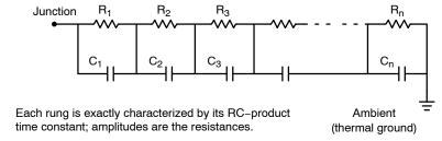
Figure 25. Non-Grounded Capacitor Thermal Ladder ("Foster" Ladder)
