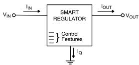
Figure 32. Single Output Regulator with Key Performance Parameters Labeled
