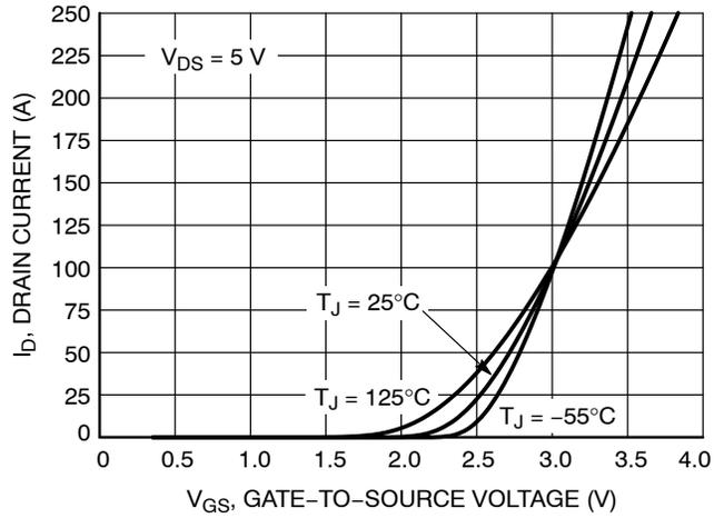
Figure 2. Transfer Characteristics
