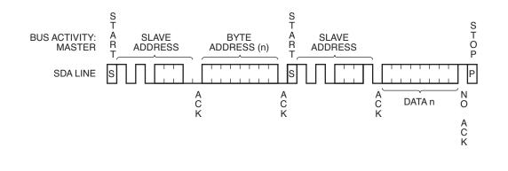
Figure 11. Sequential Read Timing
