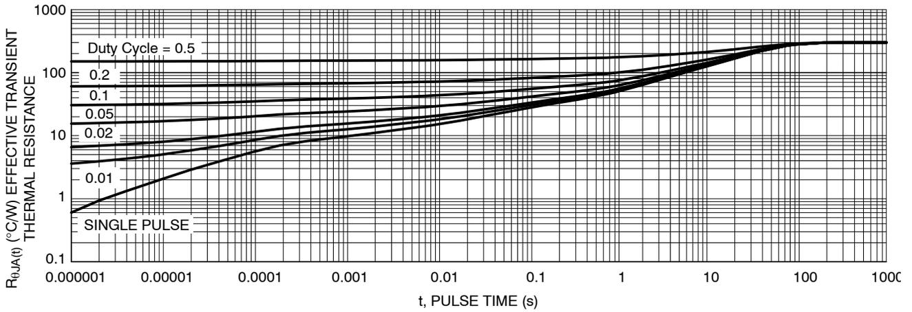
Figure 11. Thermal Response - 1 sq in pad
