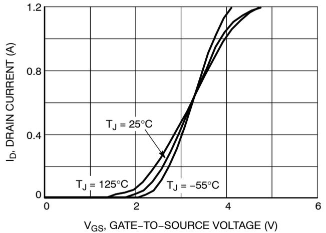
Figure 2. Transfer Characteristics
