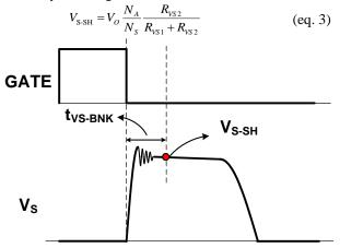
Figure 26 Output Voltage Detection
