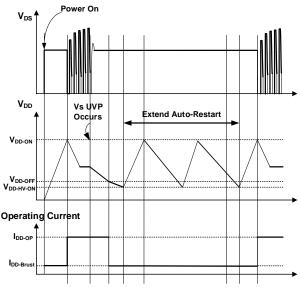
Figure 34 Extend Auto-Restart Mode Operation
