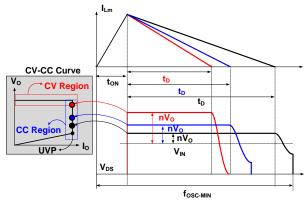
Figure 30 The Minimum Operation Frequency
