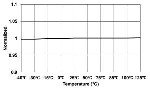
Figure 15 Current Limit Threshold Voltage (V<sub>CS-LIM</sub>) vs. Temperature
