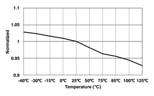
Figure 16 High Threshold Voltage of Current Sense
