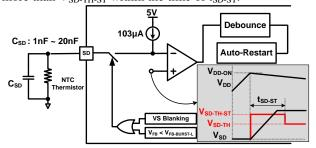
Figure 37 External OTP using SD Pin
