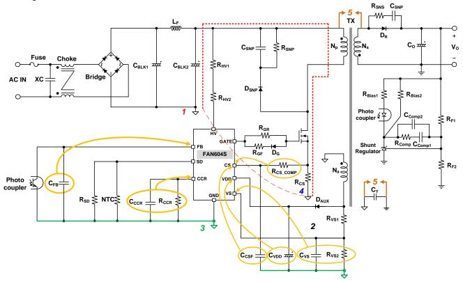
Figure 39 Recommended Layout for FAN604S
