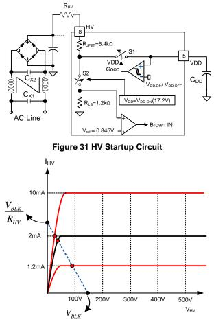
Figure 32 Characteristics of HV pin
