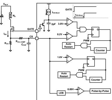
Figure 38 Current Sense Protection Circuit
