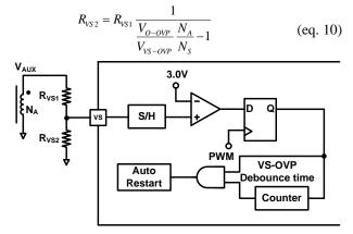
Figure 35 VS-OVP Protection Circuit
