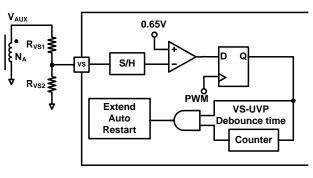
Figure 36 VS-UVP Protection Circuit
