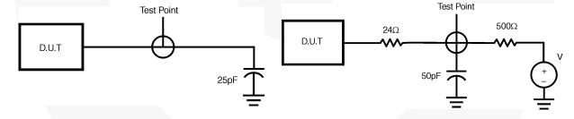
Figure 7. Load for V<sub>M</sub>/V<sub>P</sub> and RCV
