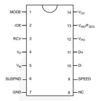
Figure 2. TSSOP and SOIC Pin Assignments
