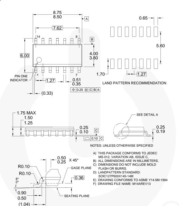
Figure 10. 14-Lead, Small Outline Integrated Circuit (SOIC) MO-012, 0.150-inch Wide
