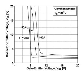
Figure 7. Saturation Voltage vs. V<sub>GE</sub>
