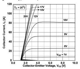
Figure 3. Typical Saturation Voltage Characteristics
