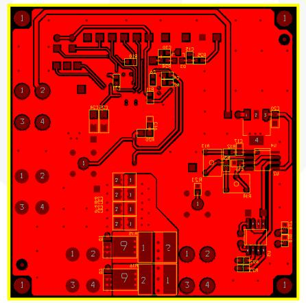
Figure 33. Evaluation Board Bottom Layer Copper
