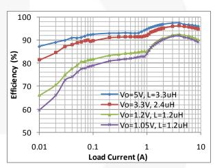
Figure 7. FAN2306A Efficiency vs. Load Current with  $$V_{\text{OUT}}$=1.2\ V$ and $f_{\text{SW}}$=500\ kHz$
