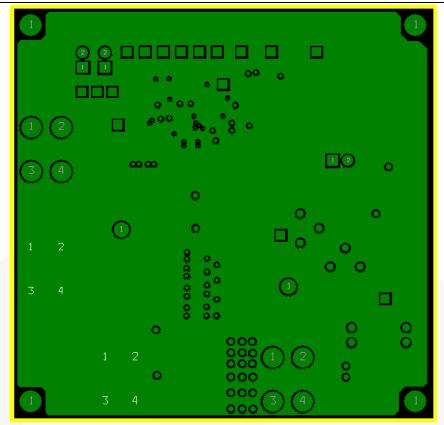
Figure 32. Evaluation Board Inner Layer 2 Copper
