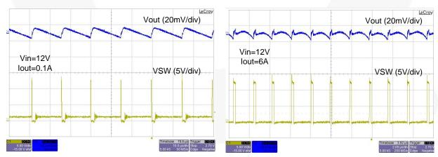
Figure 21. FAN2306A Static Output Ripple at Light Load
