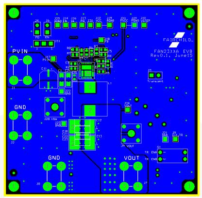
Figure 30. Evaluation Board Top Layer Copper
