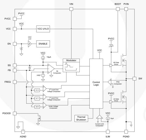
Figure 2. Block Diagram
