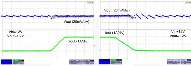
Figure 23. FAN2306A Transition from DCM to CCM
