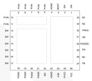
Figure 3. Pin Assignments, Bottom View
