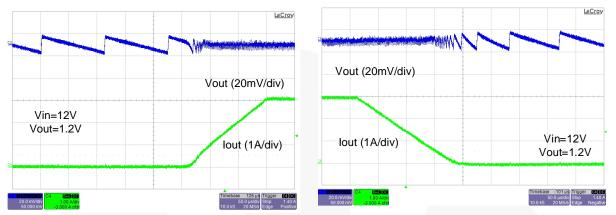
Figure 17. FAN2306MA Transition from DCM to CCM
