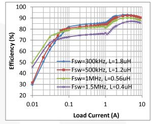
Figure 5. FAN2306A Efficiency vs. Load Current with Figure 6. FAN2306A Efficiency vs. Load Current with  $V_{IN}$ =12 V and  $f_{SW}$ =500 kHz  $V_{IN}$ =12 V and  $V_{OUT}$ =1.2 V
