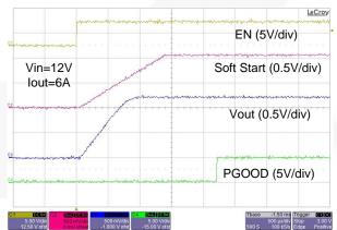
Figure 15. Startup Waveforms with 0 A Load Current Figure 16. Startup Waveforms with 6 A Load Current
