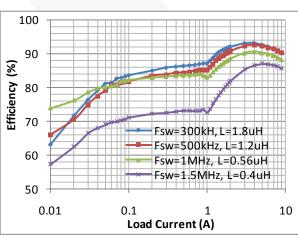
Figure 9. FAN2306MA Efficiency vs. Load Current with V<sub>IN</sub>=12 V and V<sub>OUT</sub>=1.2 V
