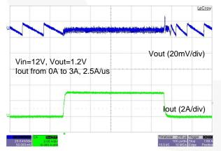
Figure 27. FAN2306MA Load Transient from 0% to 50% Load Current
