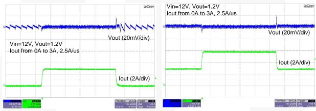
Figure 25. FAN2306A Load Transient from 0% to 50% Load Current
