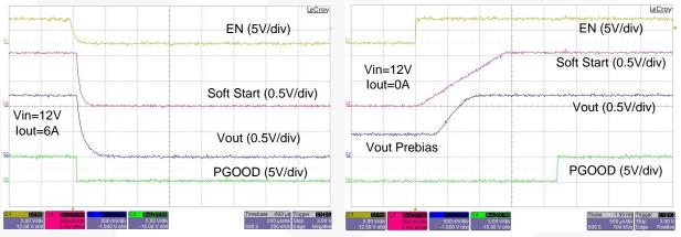
Figure 19. Shutdown Waveforms with 6 A Load Current
