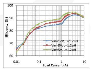
Figure 10. FAN2306MA Efficiency vs. Load Current with V<sub>OUT</sub>=1.2 V and f<sub>SW</sub>=500 kHz
