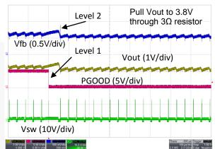
Figure 28. Over-Current Protection with Heavy Load
