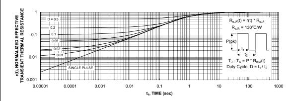
Figure 11. Transient Thermal Response Curve.
