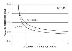
Figure 4. On-Resistance Variation with Gate-to-Source Voltage.
