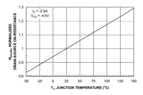
Figure 3. On-Resistance Variation with Temperature.
