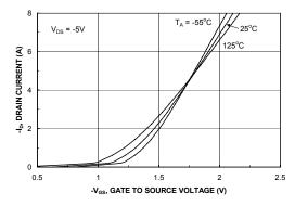
Figure 5. Transfer Characteristics.
