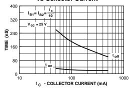
Switching Times vs Collector Current
