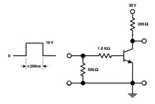
FIGURE 1: Saturated Turn-On Switching Timer
