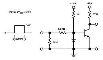
FIGURE 2: Saturated Turn-Off Switching Time
