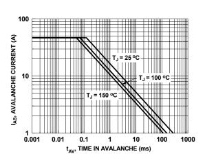
Figure 9. Unclamped Inductive Switching Capability
