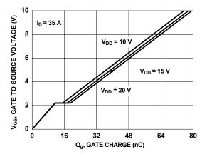
Figure 7. Gate Charge Characteristics
