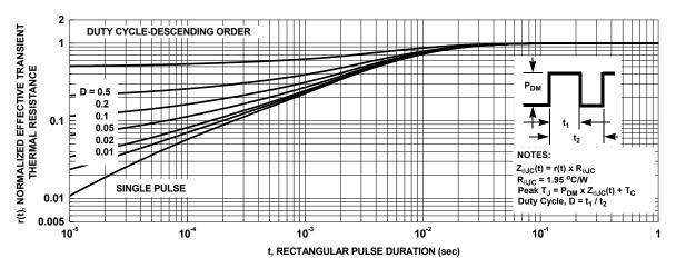
Figure 13. Junction-to-Case Transient Thermal Response Curve
