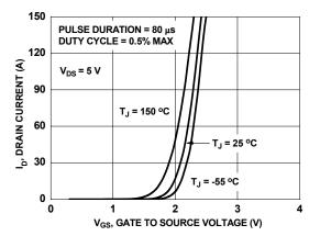
Figure 5. Transfer Characteristics
