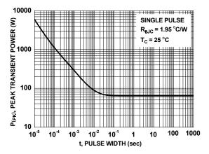
Figure 12. Single Pulse Maximum Power Dissipation
