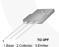
Figure 1. Pin Configuration
