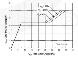
Figure 6. Gate Charge Characteristics
