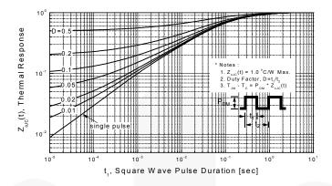
Figure 11-1. Transient Thermal Response Curve for FCP11N60
