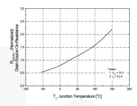
Figure 8. On-Resistance Variation vs. Temperature
