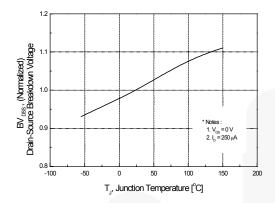
Figure 7. Breakdown Voltage Variation vs. Temperature
