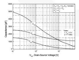
Figure 5. Capacitance Characteristics
