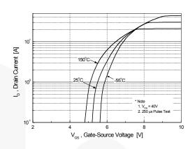
Figure 2. Transfer Characteristics
