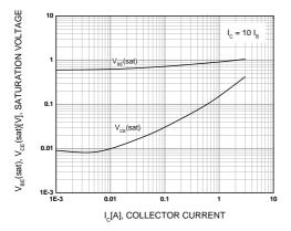
Figure 3. Base-Emitter Saturation Voltage Collector-Emitter Saturation Voltage
