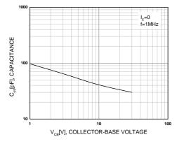
Figure 5. Collector Output Capacitance
