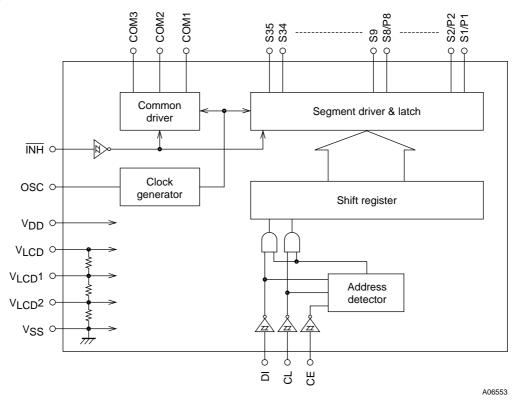
Note: The LC75833JE does not have the S12, S23, S24, S35 output pins.
