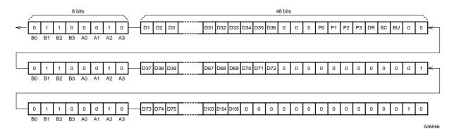
Note: At the LC75833JE, the display data D34 to D36, D67 to D72, D103 to D105 must be set to 0.
