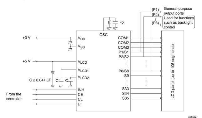
Note: \*2 When a capacitor except the recommended external capacitance (C<sub>OSC</sub> = 1000 pF) is connected the OSC pin, we recommend that applications connect the OSC pin with a capacitor in the range 220 to 2200pF.
