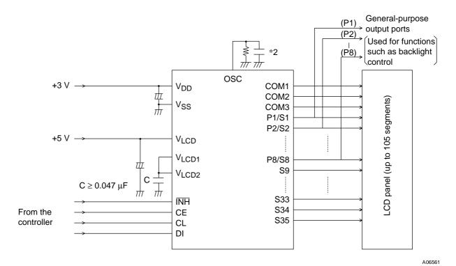
Note: \*2 When a capacitor except the recommended external capacitance (COSC = 1000 pF) is connected the OSC pin, we recommend that applications connect the OSC pin with a capacitor in the range 220 to 2200pF.
