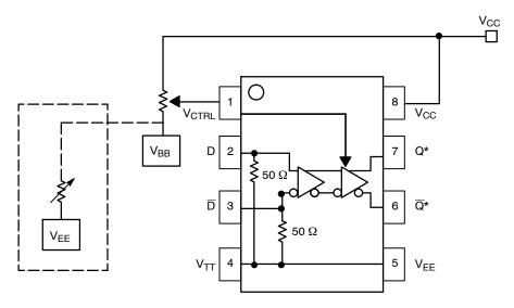
Figure 5. Alternative Implementations,  $V_{CTRL}$  Pin 1
