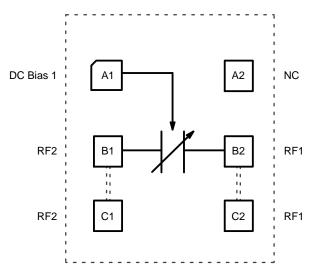
Figure 1. PTIC Functional Block Diagram (Top Level View)
