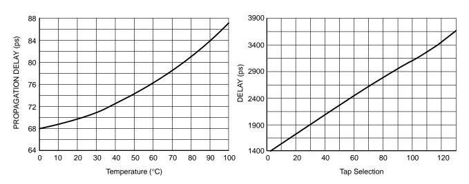
Figure 9. Delay vs. Temperature (Per Gate).
