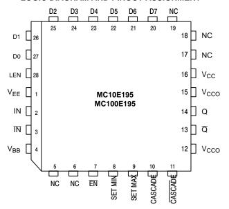
Figure 1. Pinout:28-Lead PLCC (Top View)
