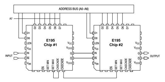
Figure 3. Cascading Interconnect Architecture
