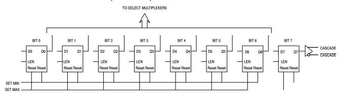
Figure 4. Expansion of the Latch Section of the E195 Block Diagram
