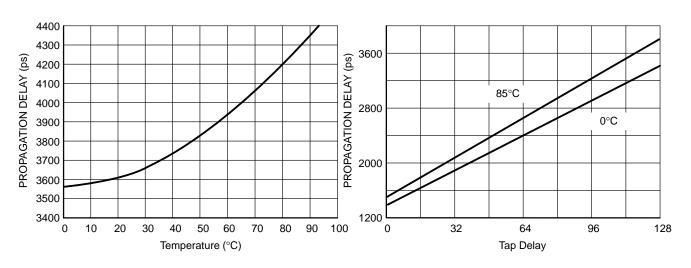
Figure 7. Delay vs. Temperature (Max. Delay).
