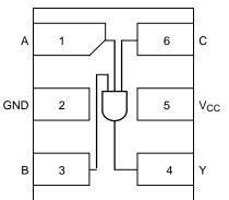
Figure 1. Pinout (Top View)
