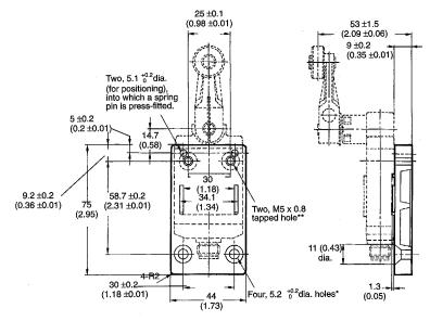
Note: Four hexagonal flat head bolts (M5 x 0.8, length: 10) and two hexagonal head bolts (M5 x 0.8, length: 15) are included. \*All the holes with 5.2+0.2/0 dia. must be used with M5 x 10 hexagonal head bolts.
