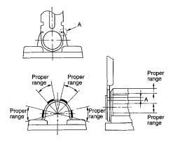
Refer to the following figure to set the stroke of a D4CC Limit Switch mounted on a panel.
