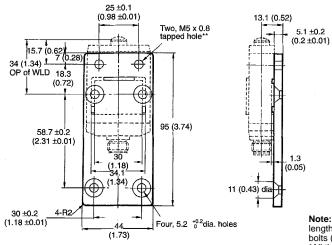
Note: Four hexagonal flat head bolts (M5 x 0.8, length: 10) and two hexagonal head bolts (M5 x 0.8, length: 15) are included.
