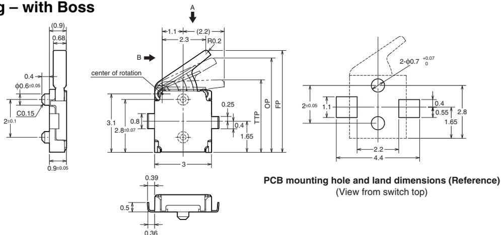
**Note:** 1. Unless otherwise specified, all units are in millimeters and a tolerance of  $\pm 0.15$  mm applies to all dimensions
