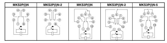
**LED Indicator Type** (DC Coil: Standard Polarity)
