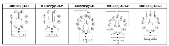
**LED Indicator and** Diode Type (DC Coil)
