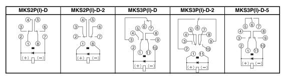
Diode Type (DC Coil: Reverse Polarity)
