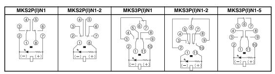
**Diode Type** (DC Coil: Standard Polarity)
