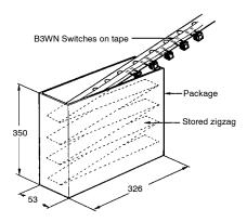
Do not press strongly, vibrate, or drop the package, otherwise the terminals of the Switches may deform.
