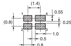
Unless otherwise specified, the dimensional tolerance is  $\pm 0.1$  mm.
