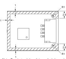
Note: Due to insulation distance limitations, do not allow metal parts to come into contact with the Sensor.
