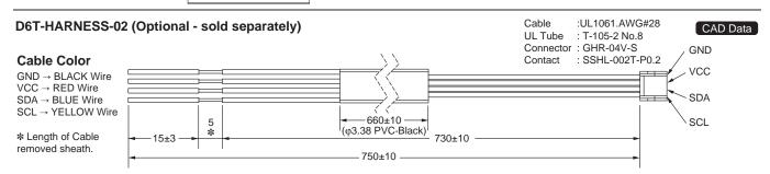
Note: Unless otherwise specified, a tolerance of  $\pm 0.3$  mm applies to all dimensions.
