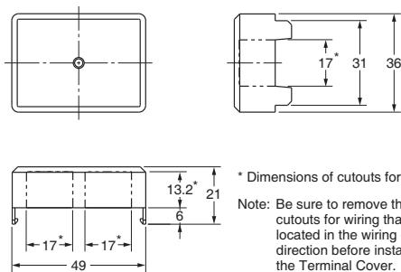
\* Dimensions of cutouts for wiring.
