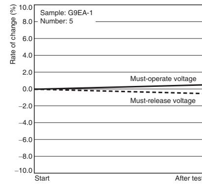
Characteristics were measured after applying a shock of 490 m<sup>2</sup>/s to the test piece 3 times each in 6 directions along 3 axes. The percentage rate of change is the average value for all of the samples.
