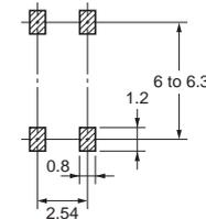
\* The external dimensions are different from those of the standard SOP 4-pin, but the mounting pad dimensions are the same.
