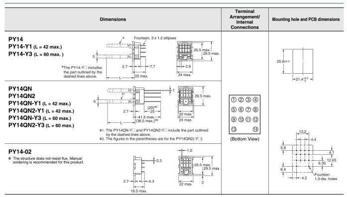
Note: 1. Use a panel with a thickness of 1 to 2 mm when mounting a Socket on it.
