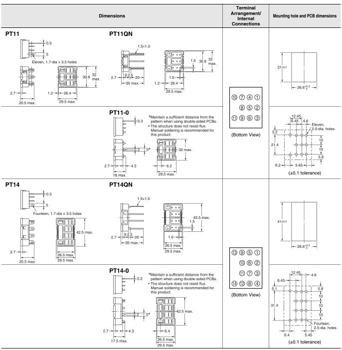
Note: Use a panel with a thickness of 1 to 2 mm when mounting a Socket on it.
