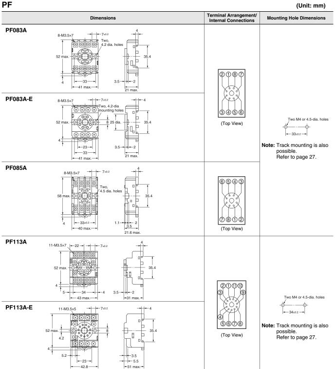
Note: 1. For the PF083A and PF113A, the Socket key slot is on the top. (Applicable model: MK)
