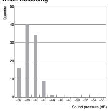
Sample: G5RL-1A-LN 12 VDC Number of relays: 100 pcs Range: A weighted sound pressure level, Fast, Max. hold
